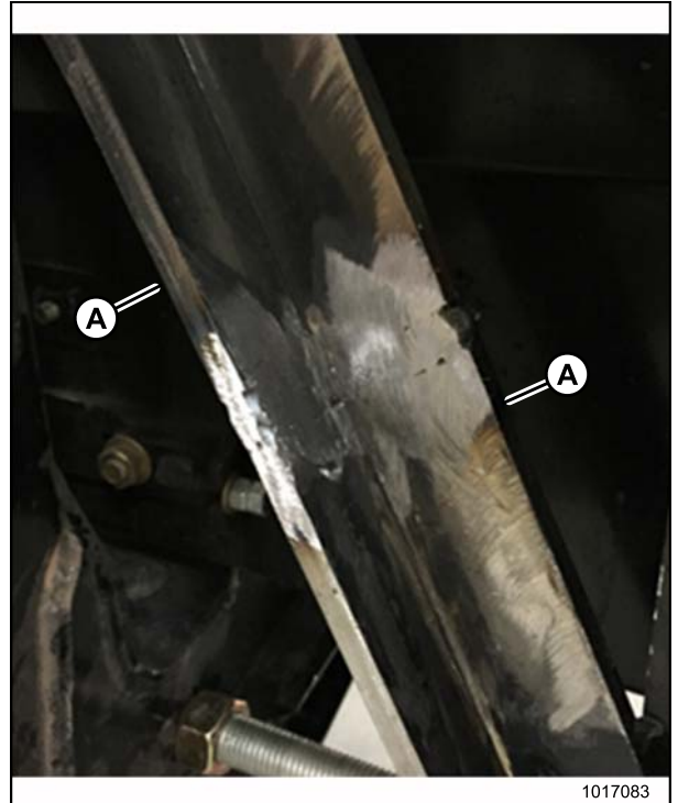
Figure 3.11: Middle Section of RH Center Frame Brace
