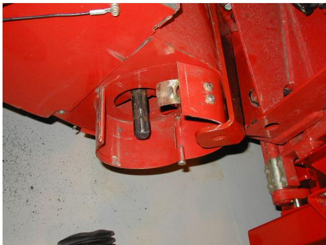
If this access for installing corn head driveline is deemed not acceptable then following rework to combine shield is required. The outer shield is made up of the two half shields with one welded to combine. Mark location of shields. Then grind off the two welds securing half shield. Rotate shield 90° counterclockwise and weld shield back on.
