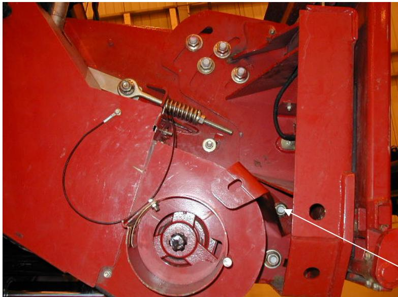
The washer between flange nut and feeder house face plate are replaced with 174216.
