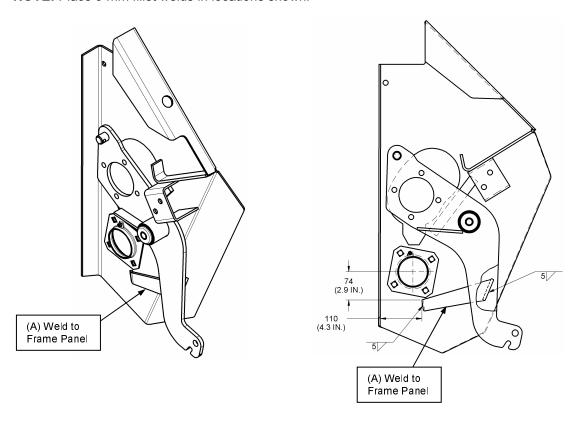
2. Position front R/H roll arm stop (B) and rear R/H roll arm stop (C) between frame panel and roll arm as shown.
