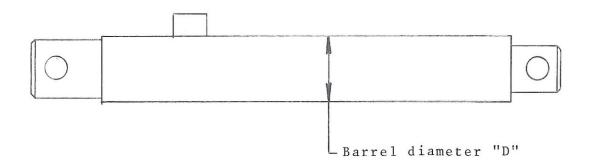
If "D" is 2 3/8 inches (60.3 mm) use Repair Parts in seal kit P-30037.
