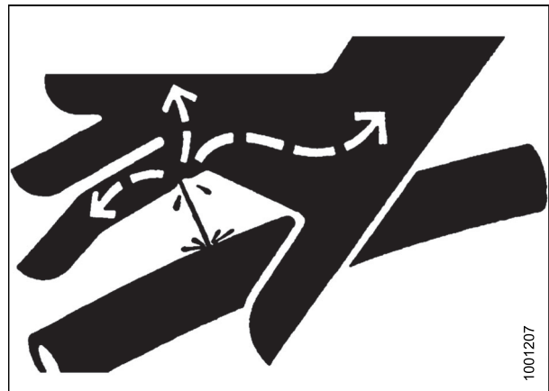
Figure 1.12: Hydraulic Pressure Hazard
