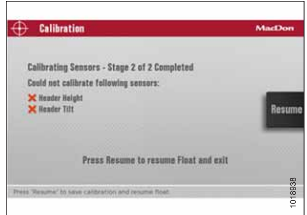
Figure 3.16: Sample of Failed Calibration Display Message
