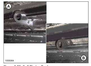
Figure 3.72: Roll Timing Tool
