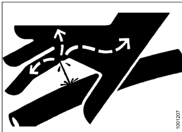
Figure 5.3: Hydraulic Pressure Hazard
