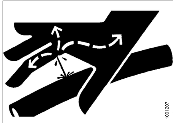
Figure 5.3: Hydraulic Pressure Hazard
