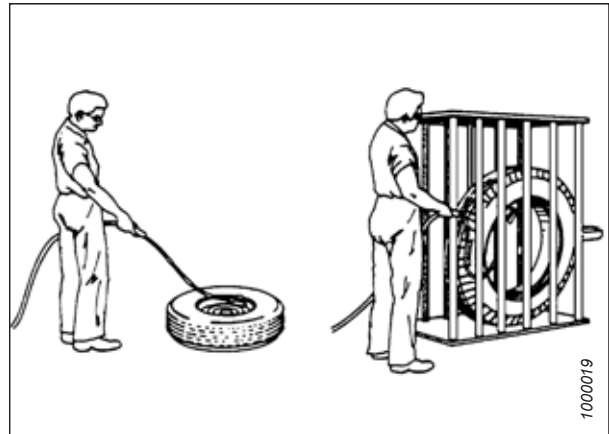
Figure 1.12: Safely Inflating Tire
