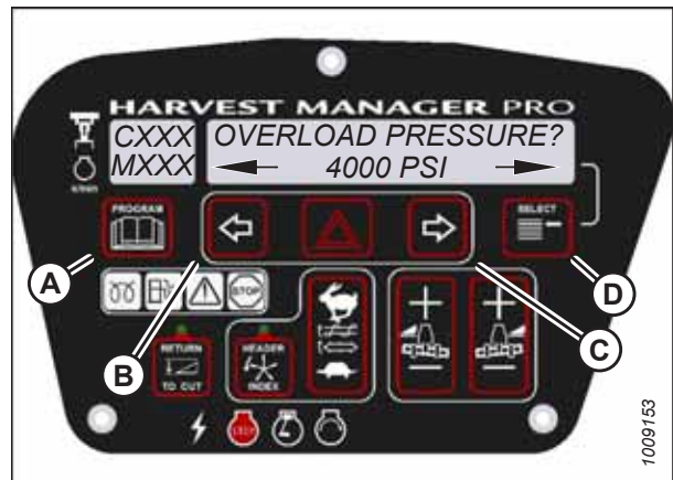
Figure 7.24: Hydraulic Overload Pressure
