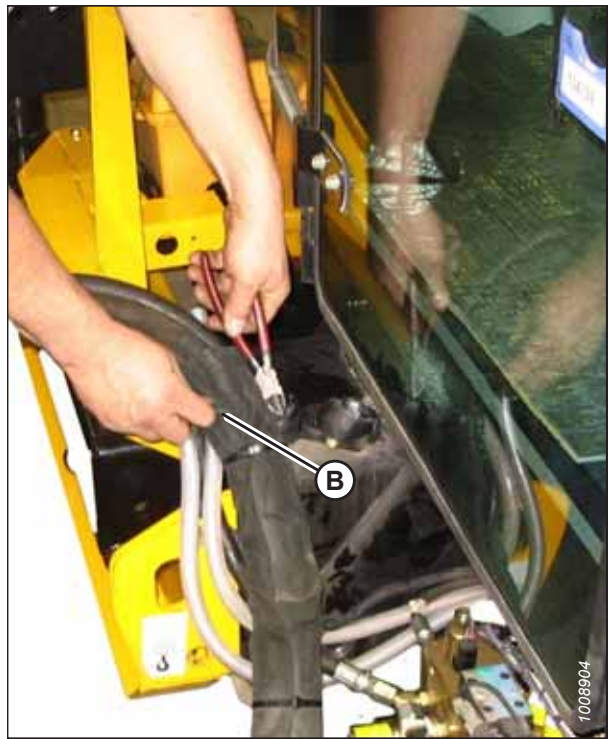
Figure 2.13: Hose Bundles on Frame
