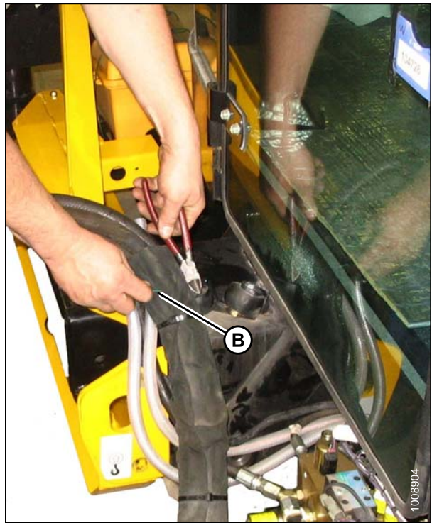
Figure 2.13: Hose Bundles on Frame
