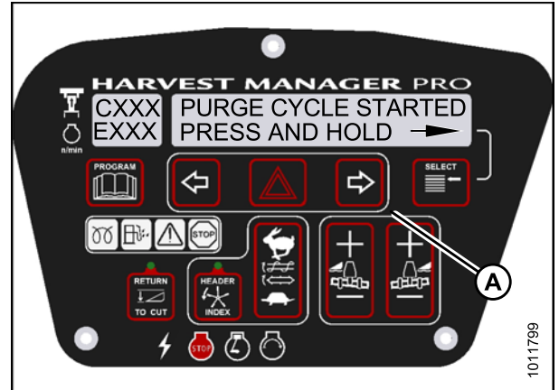
Figure 4.124: Hydraulic Purge Cycle
