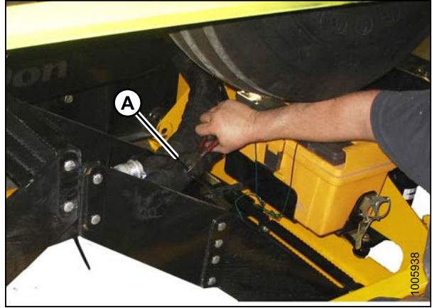
Figure 2.12: Hose Bundles on Frame
