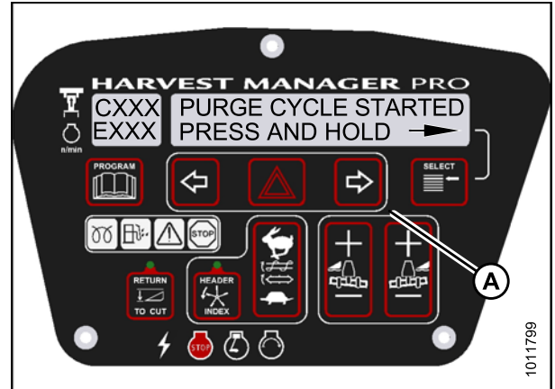
Figure 4.124: Hydraulic Purge Cycle
