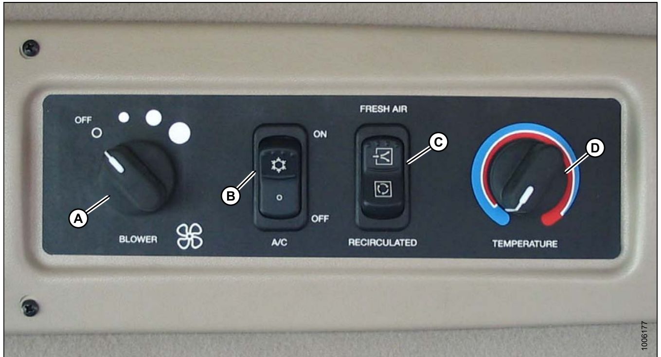
Figure 5.28: M155E4 A/C and Heater Controls
