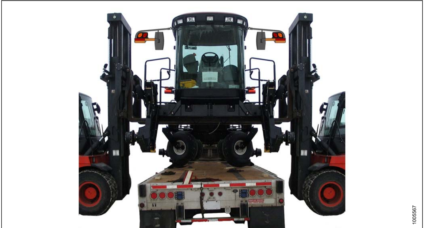
Figure 2.1: Two-Forklift Unloading Method
