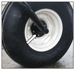
FORMED CASTER WHEEL BEARING 1 PLACE (BOTH WHEELS)
