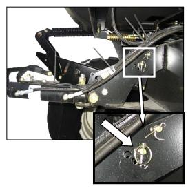
1. Re-locate the pin at the frame linkage as required to position the hook over the header
