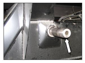
d. Adjust jack height while observing pin position in bore. When pin is loosest, tap out pin with hammer or use tool to extract pin.
