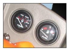
a. Check engine temperature gauge and fuel gauge are working.
