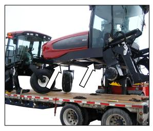
c. Position forklift on left or right side of trailer, and position forks under windrower frame.
