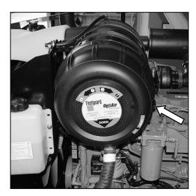
a. Check that air cleaner cap is firmly attached, and that all clamps are secure.
