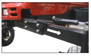
c. Slide extensions outboard equal amounts, and align holes at desired location.
