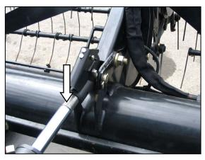
Push down on rod end of link cylinder until hook engages pin on header, and is locked. (continued next page)
