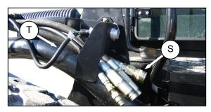
Connect header drive hoses (S) and electrical harness (T) to header. Refer to the Draper Header Operator's Manual.
