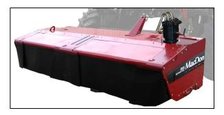
The R80 and R85 13 FT headers are shipped without the motor and hoses installed, and the installation of a separate motor and hose bundle is necessary.
