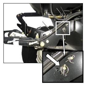
Re-locate the pin at the frame linkage as required to position the hook over the header pin.
