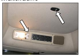
Switch lights ON and OFF with switches on each light. Interior lights only work with ROAD or FIELD light switch ON.
