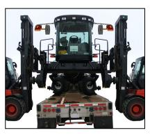
c. Position one forklift on either side of trailer, and position forks under windrower frame.
