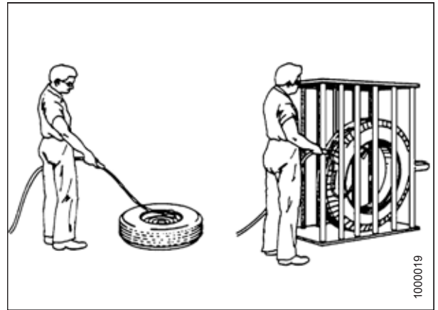
Figure 1.15: Safely Inflating Tire
