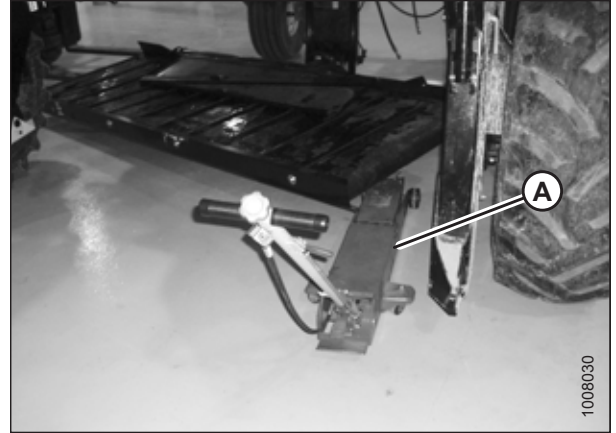
Figure 2.18: DWA Deck Supported with Floor Jack
