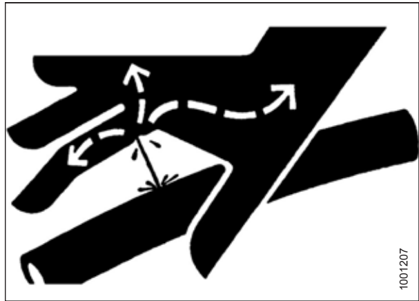
Figure 1.12: Hydraulic Pressure Hazard
