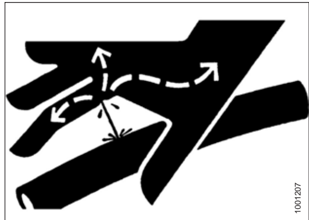
Figure 1.12: Hydraulic Pressure Hazard
