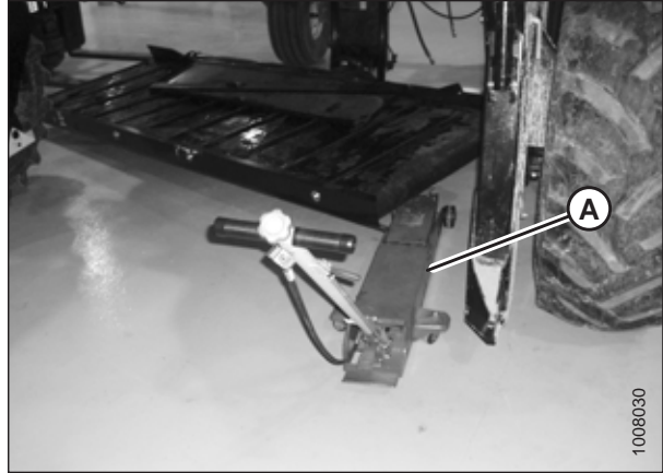
Figure 2.18: DWA Deck Supported with Floor Jack
