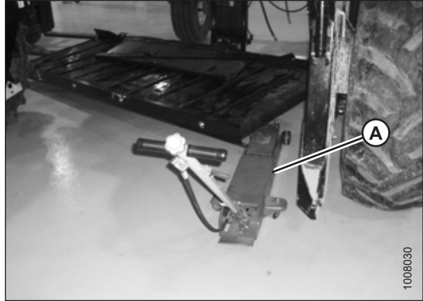
Figure 2.18: DWA Deck Supported with Floor Jack
