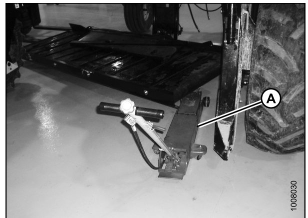
Figure 2.13: DWA Deck Supported with Floor Jack
