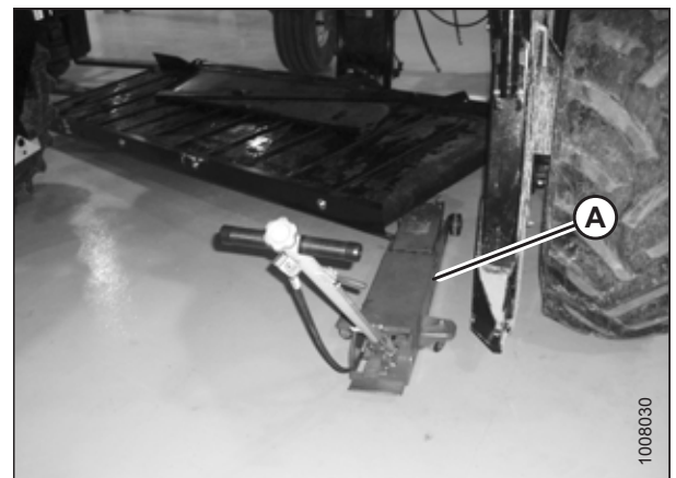
Figure 2.50: DWA Deck Supported with Floor Jack
