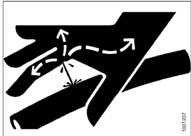
Figure 1.12: Hydraulic Pressure Hazard
