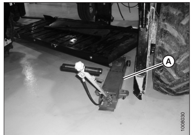
Figure 2.50: DWA Deck Supported with Floor Jack
