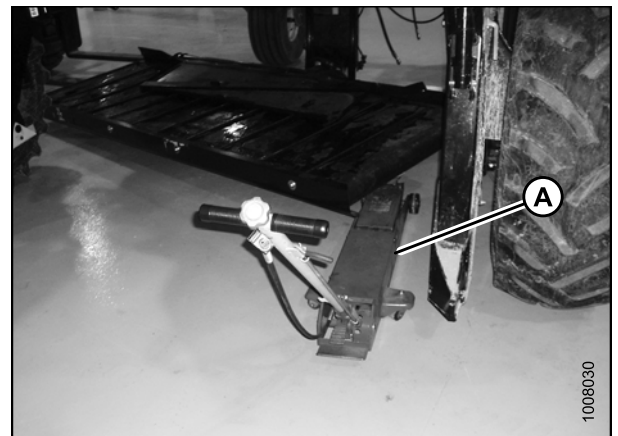
Figure 2.50: DWA Deck Supported with Floor Jack
