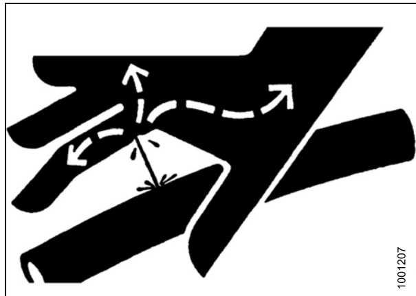
Figure 1.12: Hydraulic Pressure Hazard
