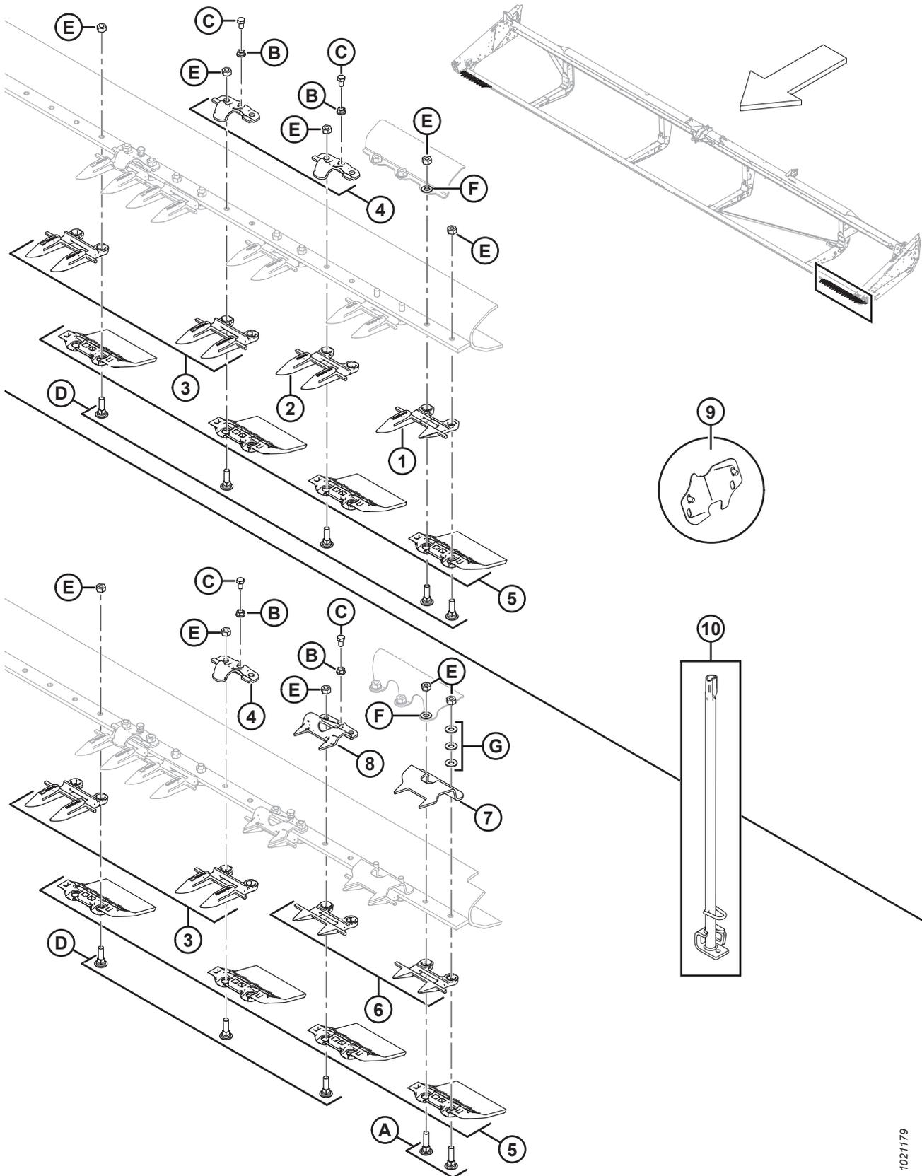
**GUARDS, HOLD-DOWNS, AND WEARPLATES – SINGLE KNIFE, POINTED AND POINTED WITH END STUBS**
