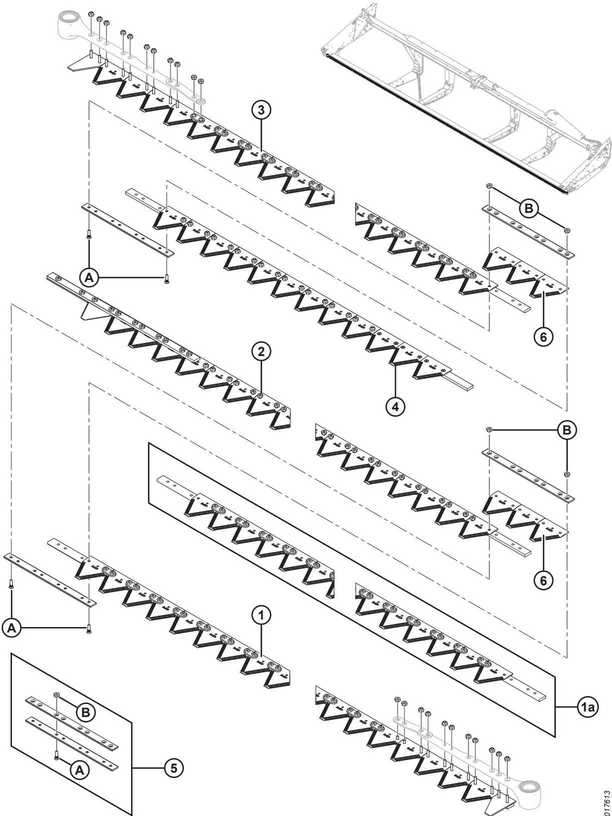
**SEGMENTED KNIVES – DOUBLE-KNIFE HEADERS, FINE-TOOTH SECTIONS**
