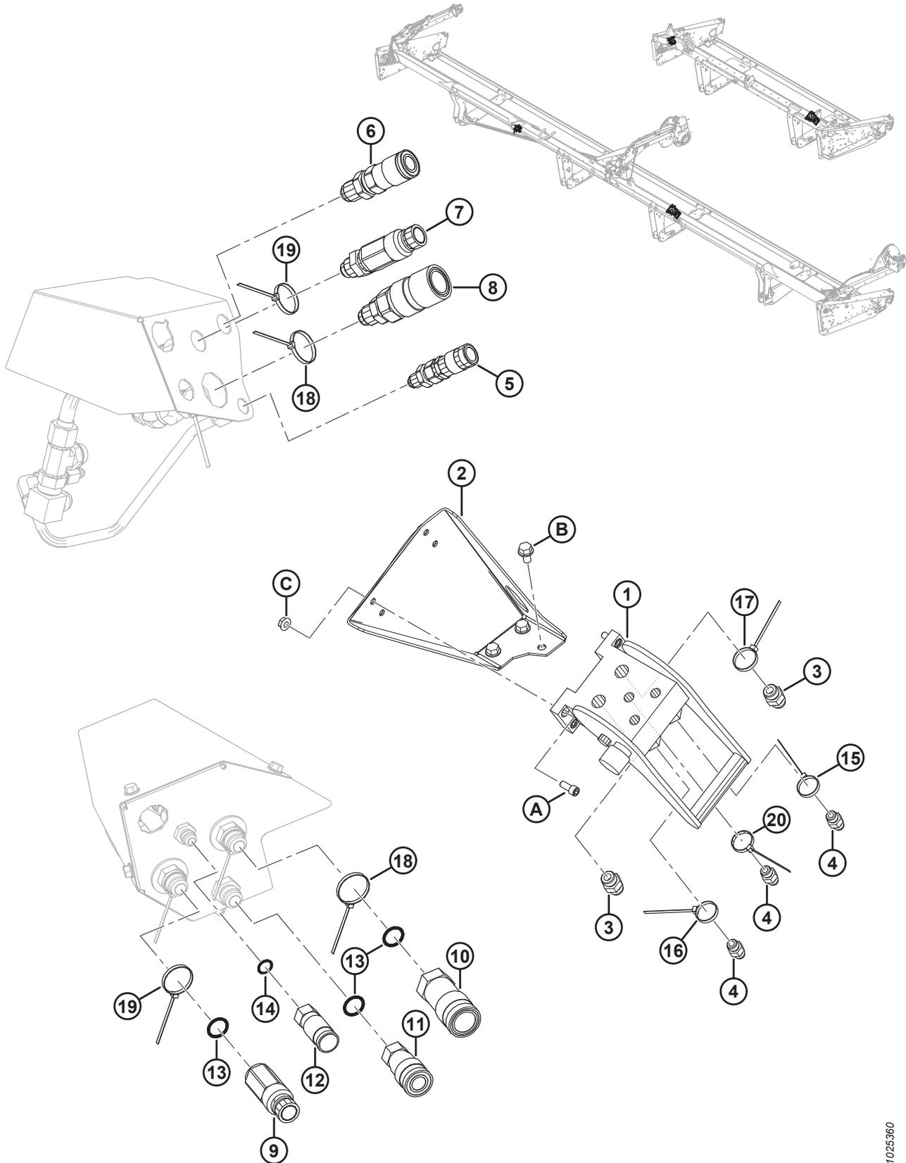
(OPTION) D1 COMPLETION PACKAGE FOR M SERIES WINDROWERS – HYDRAULIC COMPONENTS
