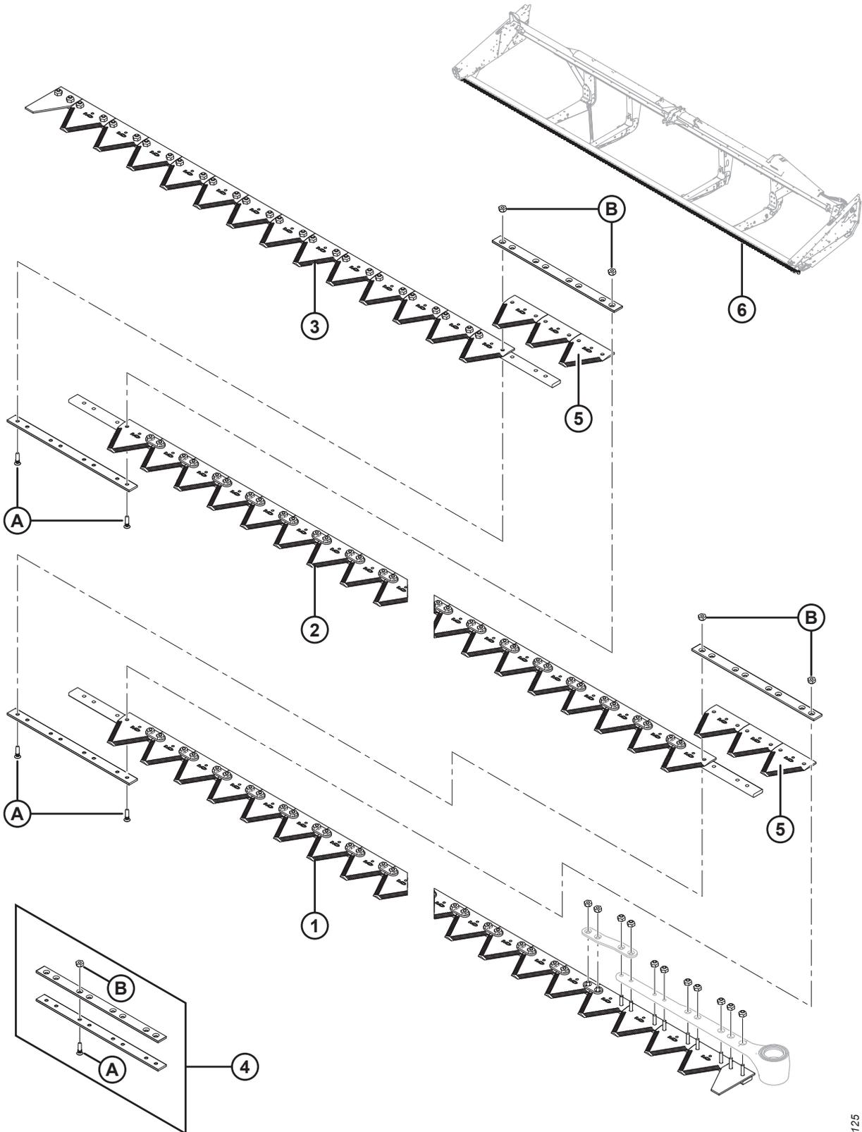
**SEGMENTED KNIVES – SINGLE-KNIFE HEADERS, COARSE-TOOTH SECTIONS**
