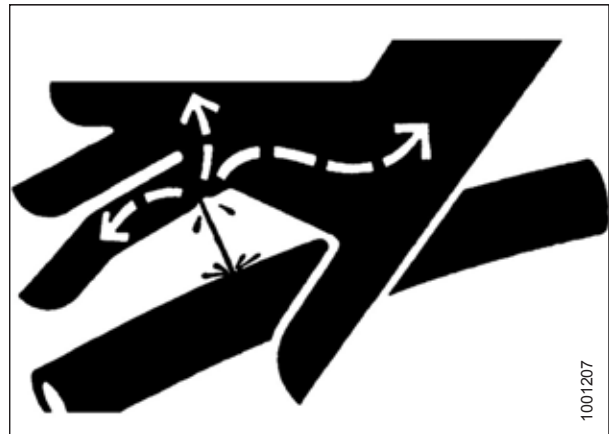
Figure 1.12: Hydraulic Pressure Hazard
