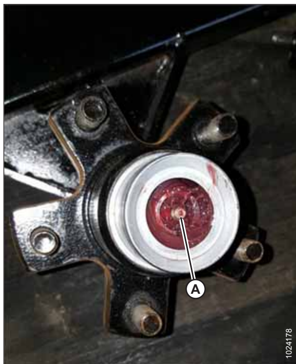
Figure 4.3: Lubrication Point on Wheel Axle
