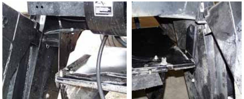
MOUNT SHIELD ON TRACTOR PINS
