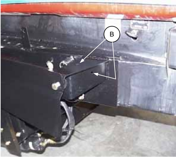
GREASE GUN HOLDER MOUNTING HOLE
