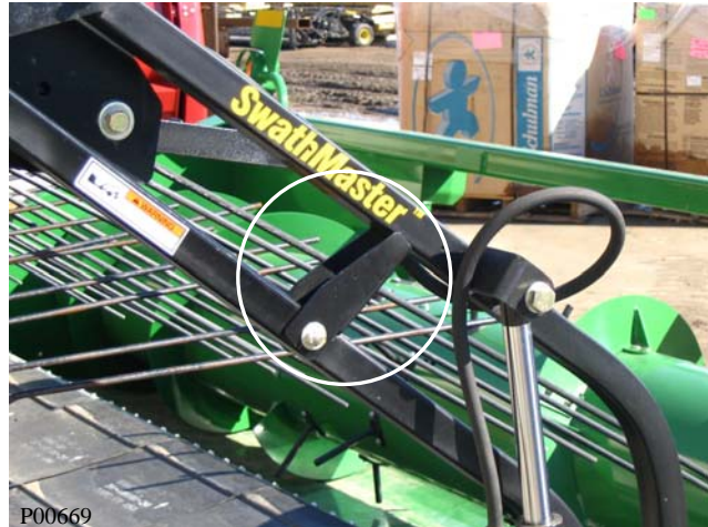
Safety Lock Engaged
