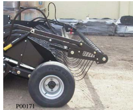
Hold-down Adjusted for Short Crops
