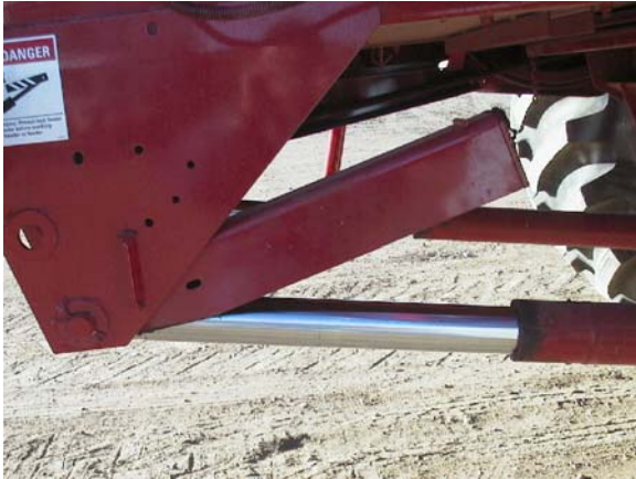
Disengaged Feeder House Lock (May not be exactly as shown)
