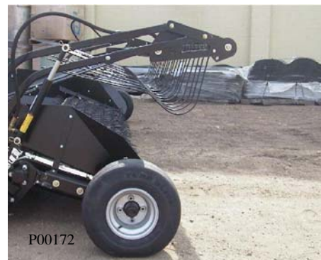
Hold-down Adjusted for Average Crops
