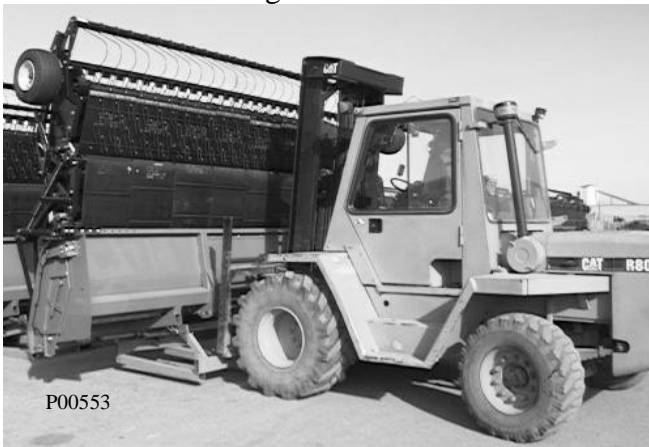
Lifting Header/Pickup In Shipping Position
