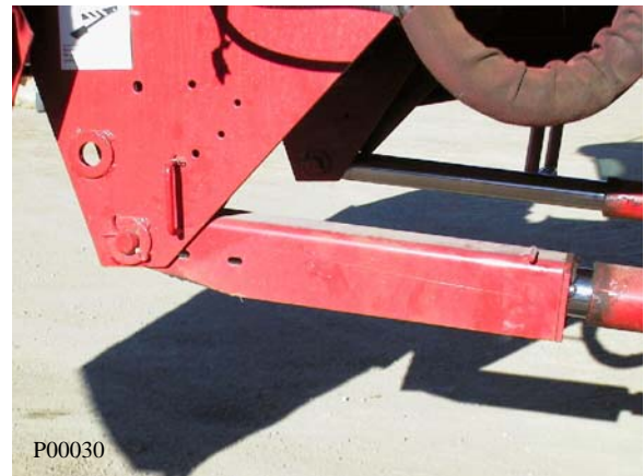
Engaged Feeder House Lock (May not be exactly as shown)
