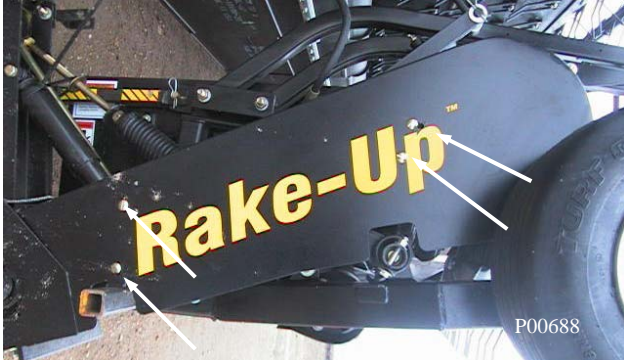
Rake-Up Drive Shield Removal
