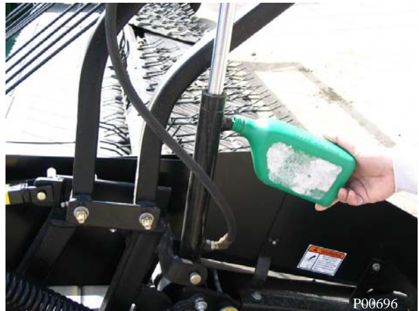
Bleeding of Hydraulics
