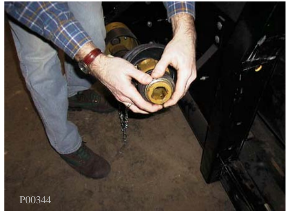
Drive Shaft to Header Installation
