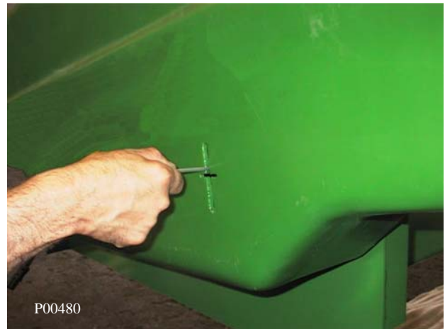
Checking Chain Tension
