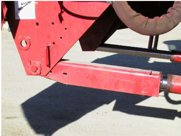
Feeder House Lock Engaged (May not be exactly as shown)
