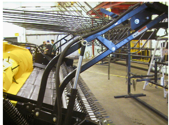
Safety Lock Engaged
