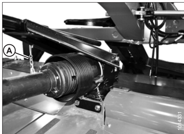
Figure 3.55: Blindage de la transmission
