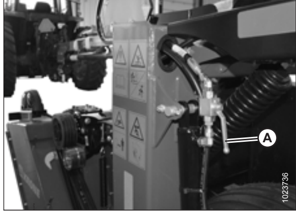
Figure 9.3: Lift Cylinder Lock-Out Valve in Open Position
