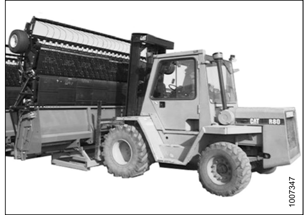
Figure 3.2: Unloading the Header
