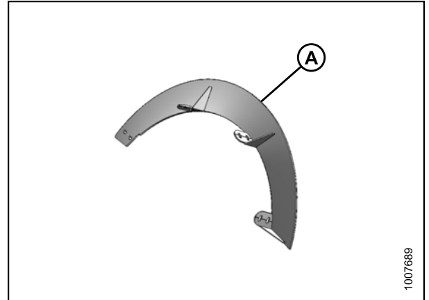
Figure 4.45: Left Extension – Right Opposite
