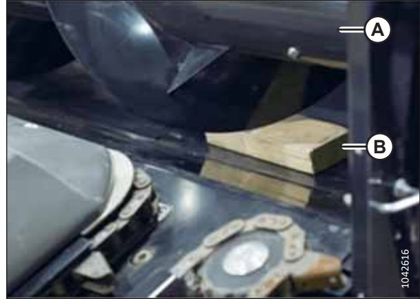
Figure 5.12: Auger Resting on Wood Block
