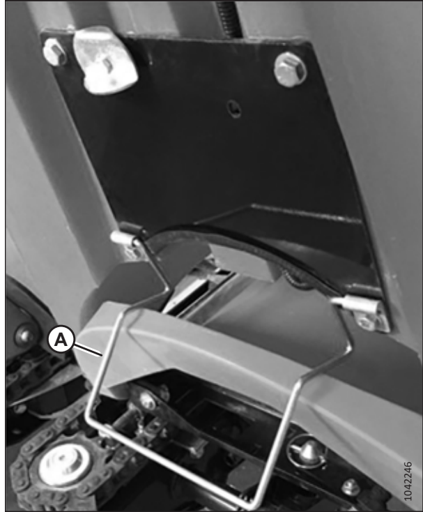
Figure 4.39: Wire Bracket Support Installed on Front Snout – Raised Service Position
