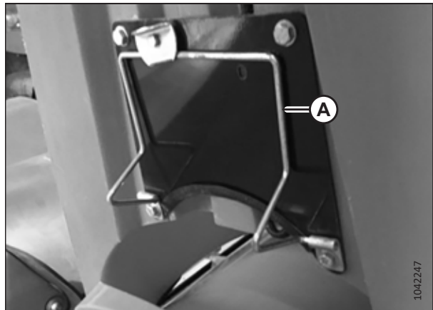
Figure 4.40: Wire Bracket Support Installed on Front Snout – Field Position
