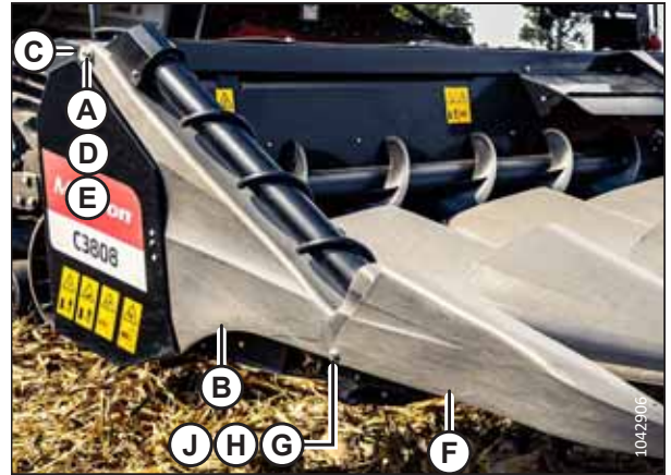
Figure 4.31: RED Installed on Header – Right Side
