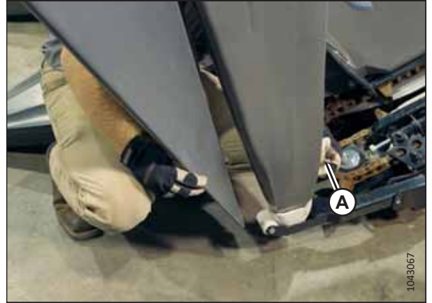
Figure 4.35: TED Installed on Left Standard End Divider
