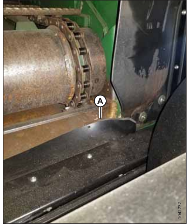
Figure 4.15: Too Large Transition Frame Seal
