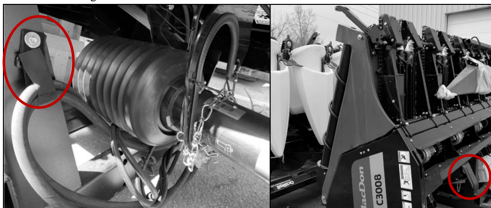
Figure 2: Velcro straps securing bulkhead lines (left), header field stands (right).
