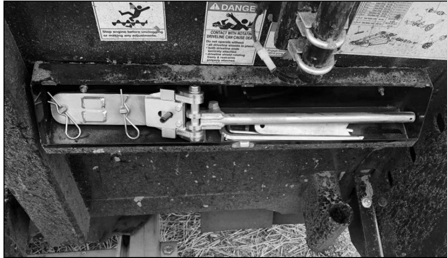
Figure 24: Tools stored in header toolbox.
