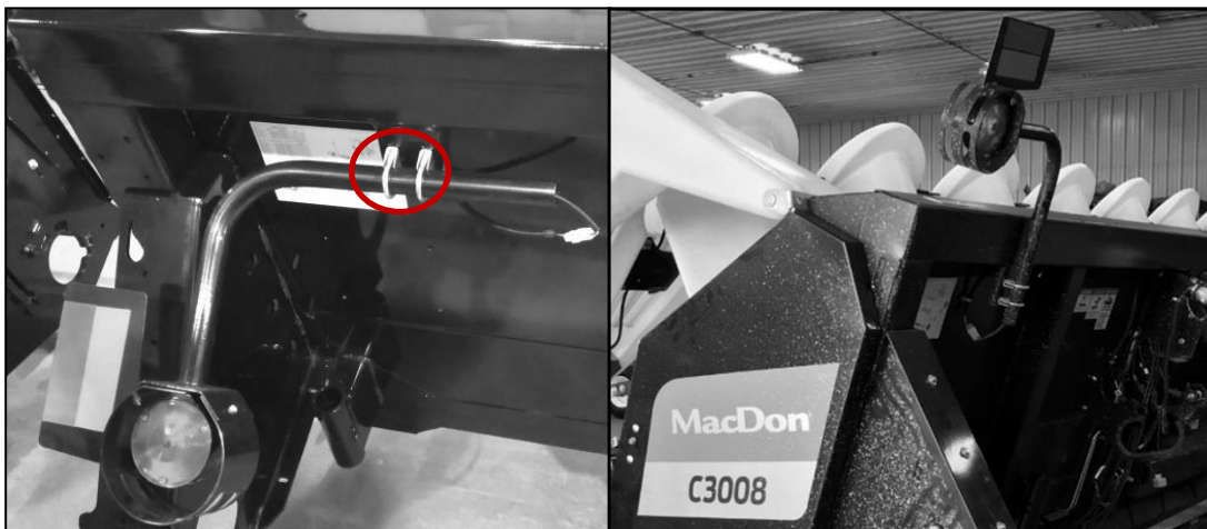
Figure 5: Clearance light secured by U-bolts (red circle, left) in shipping position (left) and field position (right).
