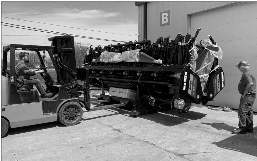
Figure 8: Removing header from header cart.
