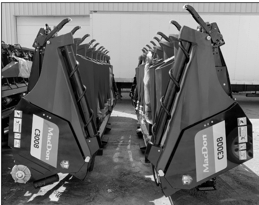
Figure 16: Orientation of headers when placed on trailer for shipping.
