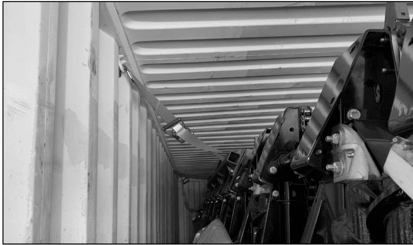
Figure 1: Ratchet straps securing header to container.
