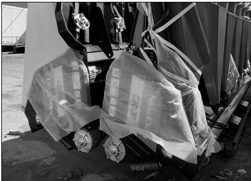
Figure 15: Bubble shipping packaging protecting auger doors needing to be removed after removing header from container.
