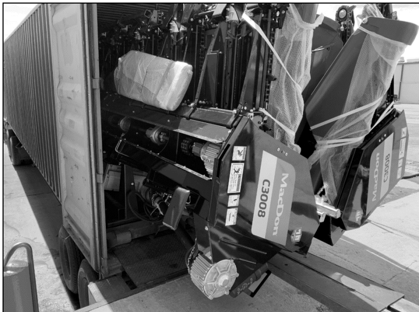
Figure 4: Removing header cart from container.
