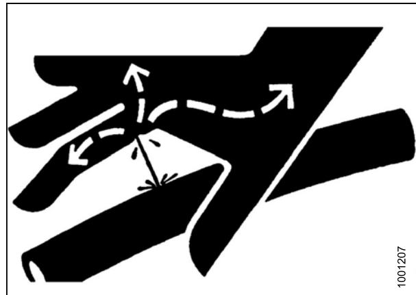
Figure 1.12: Hydraulic Pressure Hazard
