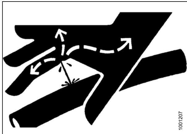
Figure 1.12: Hydraulic Pressure Hazard
