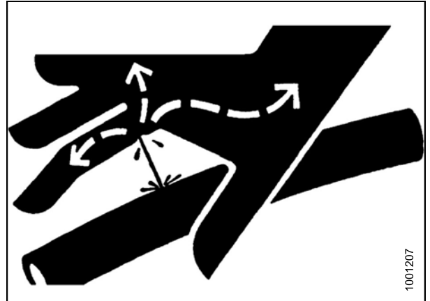
Figure 5.75: Hydraulic Pressure Hazard
