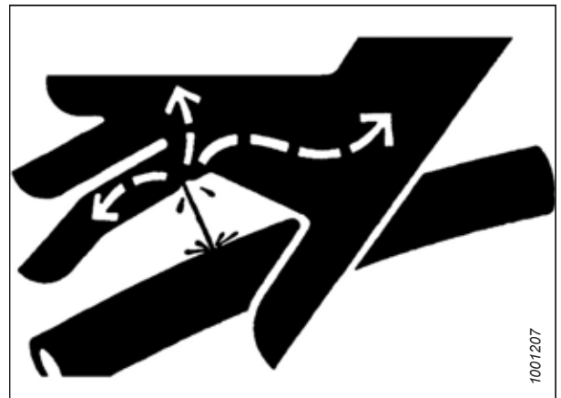
Figure 4.220: Hydraulic Pressure Hazard
