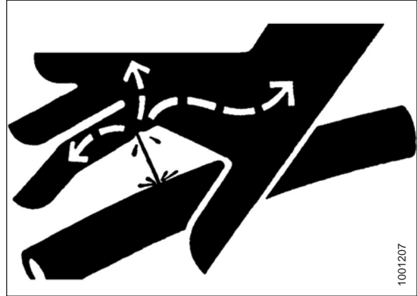
Figure 4.196: Hydraulic Pressure Hazard
