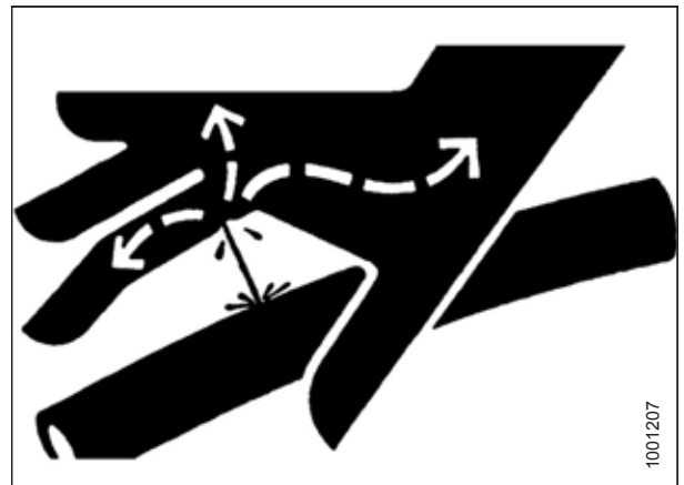
Figure 4.310: Hydraulic Pressure Hazard
