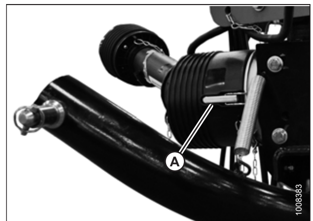
Figure 4.213: Driveline Shield Cone and Lever Clamp
