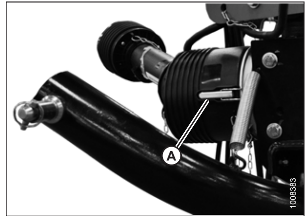
Figure 4.217: Shield Clipped to Driveline
