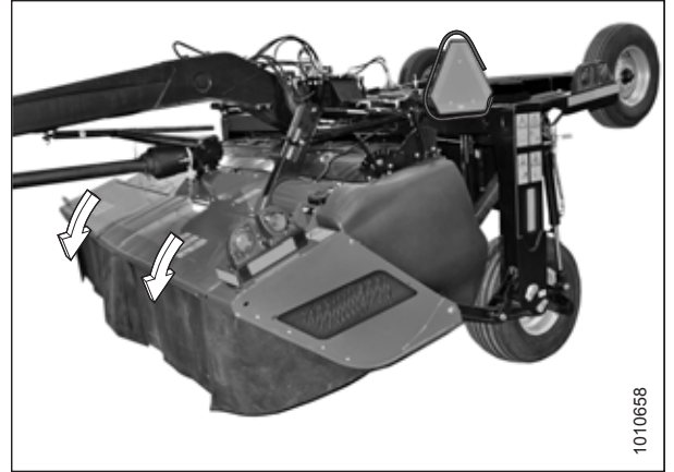
Figure 3.145: Cutterbar Doors in Closed Position
