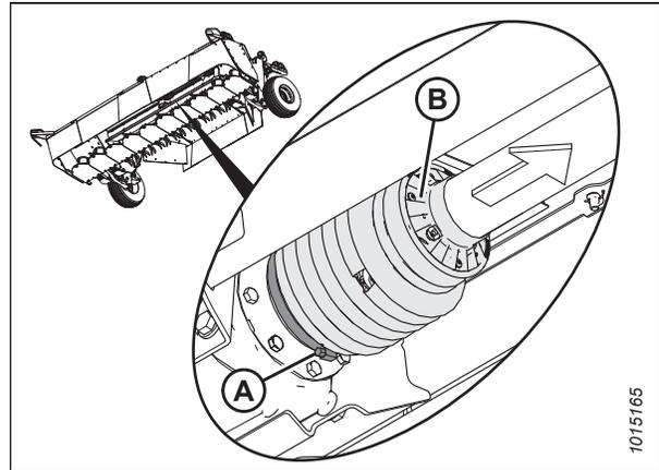
Figure 4.261: Protection de la transmission transversale
