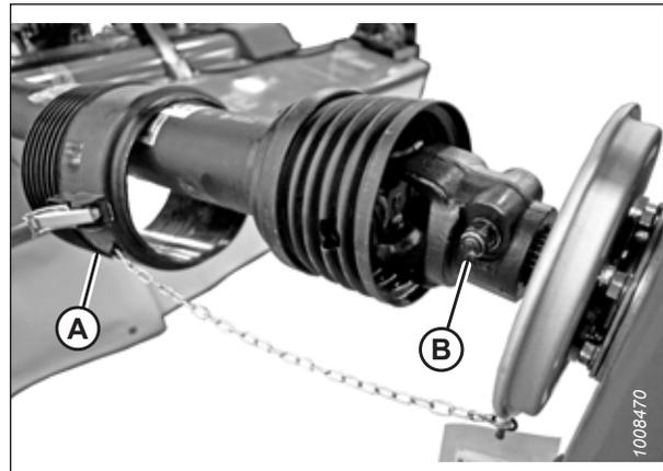
Figure 4.244: Joint universel
