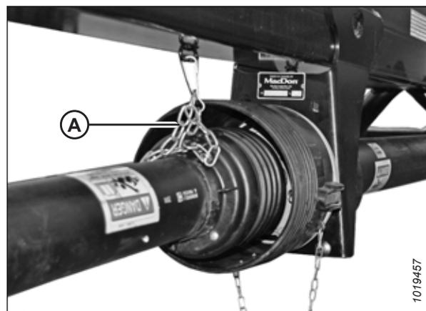
Figure 4.234: Protection de transmission
