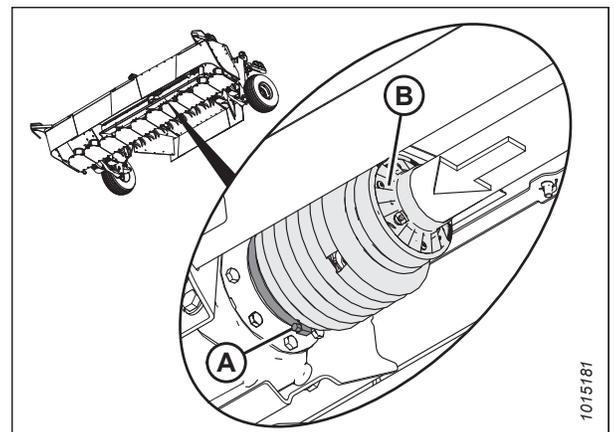
Figure 4.265: Soufflet de protection de la transmission transversale
