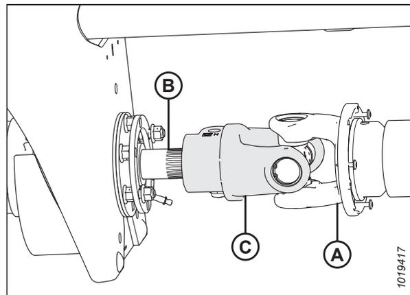
Figure 4.250: R113 PT Transmission de l'embrayage
