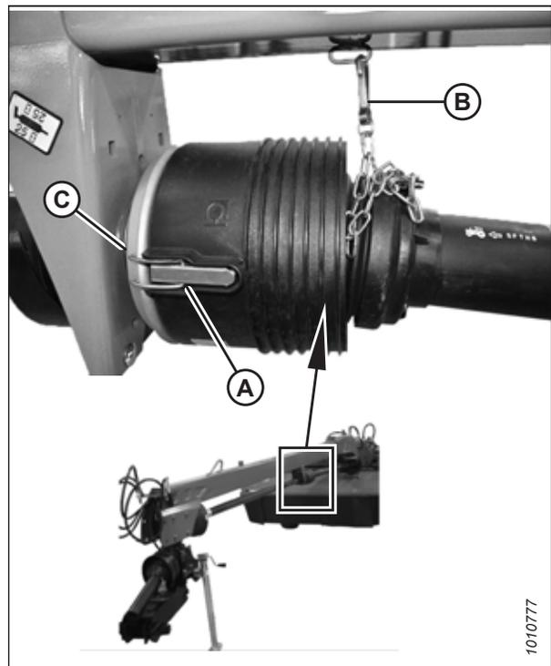
Figure 4.254: Cône de protection de la transmission
