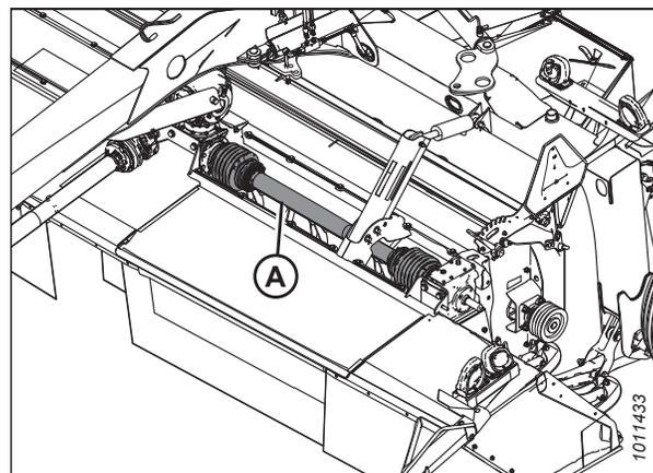
Figure 4.259: Transmission transversale
