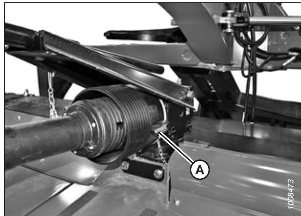
Figure 4.258: Cône de protection de la transmission
