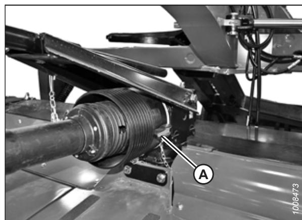
Figure 4.255: Cône de protection de la transmission
