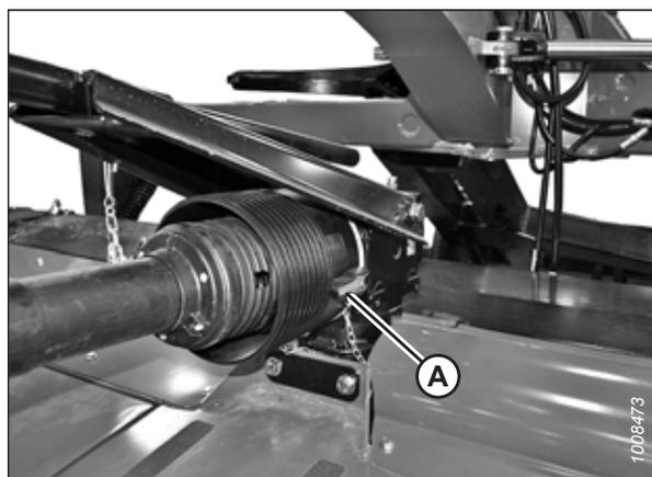
Figure 4.249: Cône de protection de la transmission
