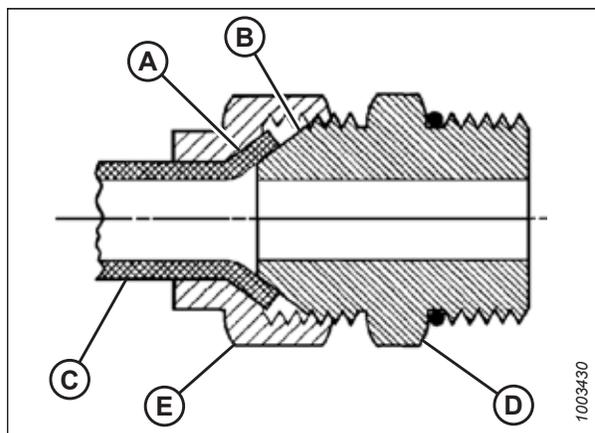
Figure 7.10: Raccord hydraulique
