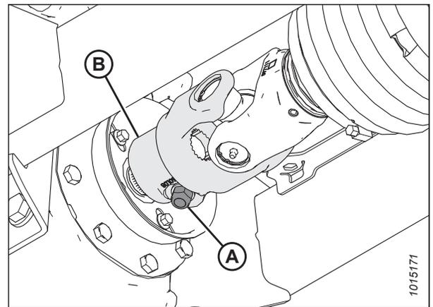
Figure 4.264: Fourche de la transmission transversale
