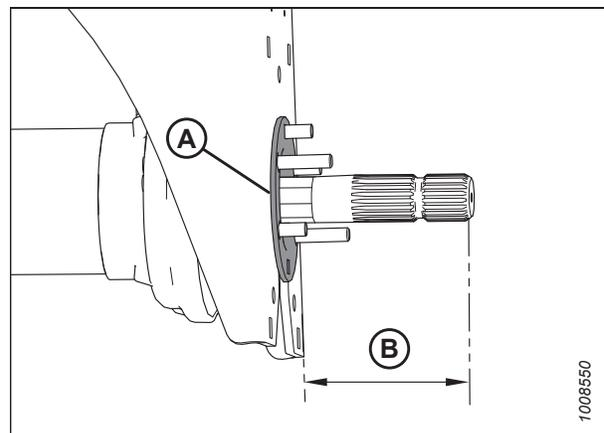
Figure 4.236: Bride installée sur le support central
