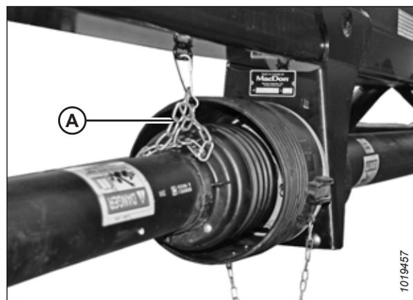
Figure 4.276: Protection de transmission
