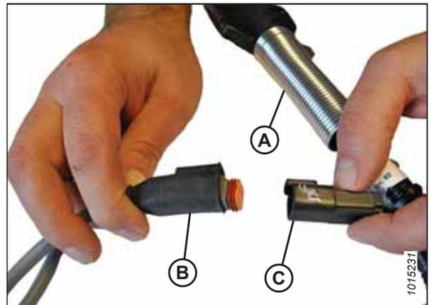
Figure 3.35: Faisceau de transport
