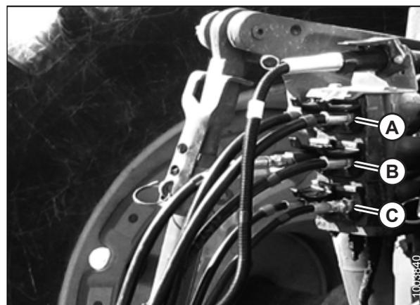
Figure 3.34: Raccords hydrauliques
