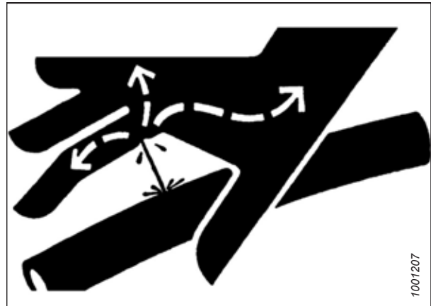
Figure 4.217: Hydraulic Pressure Hazard
