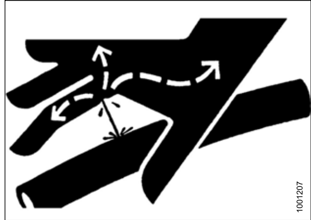
Figure 4.191: Hydraulic Pressure Hazard
