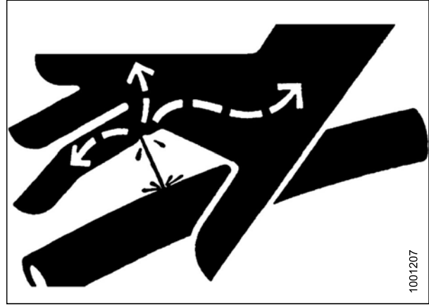
Figure 4.230: Hydraulic Pressure Hazard
