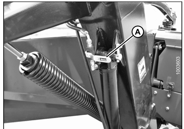
Figure 4.294: Lift Cylinder Lock-Out Valves
