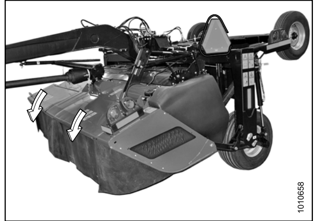
Figure 4.117: Cutterbar Doors in Closed Position
