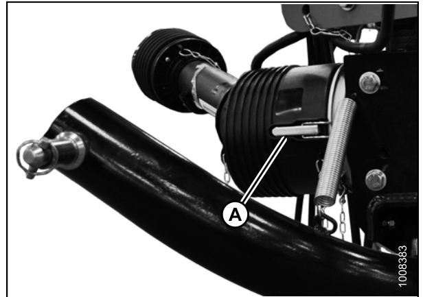
Figure 4.148: Driveline Shield Cone and Lever Clamp
