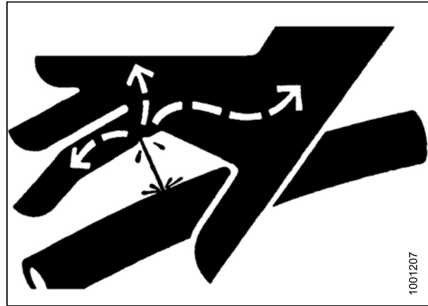
Figure 4.235: Hydraulic Pressure Hazard
