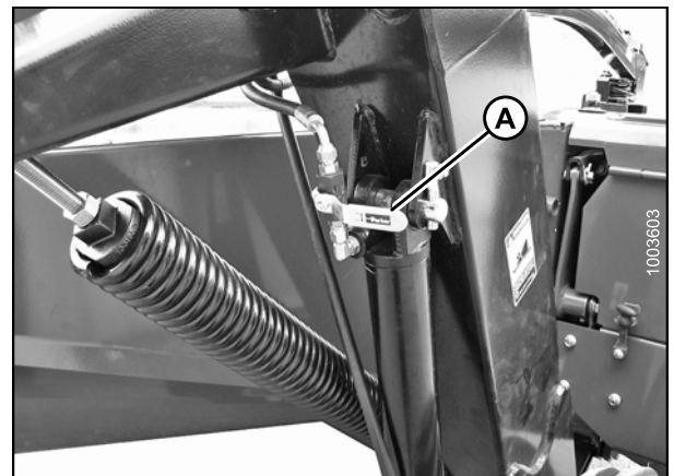
Figure 4.299: Lift Cylinder Lock-Out Valves
