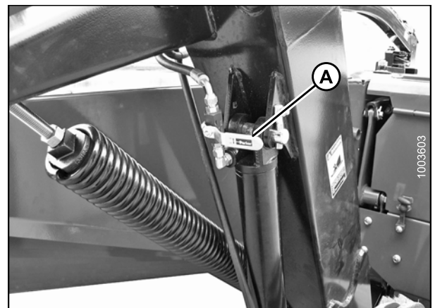
Figure 3.2: Lift Cylinder Lock-Out Valve
