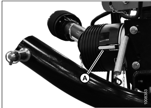
Figure 4.151: Shield Clipped to Driveline
