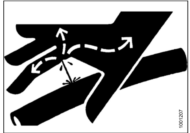
Figure 4.234: Hydraulic Pressure Hazard
