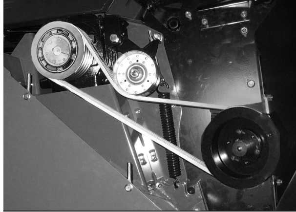
Figure 3.113: Drive Belt and Pulleys on Left Side of Conditioner
