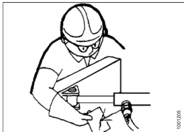
Figure 1.11: Test de fuites hydrauliques
