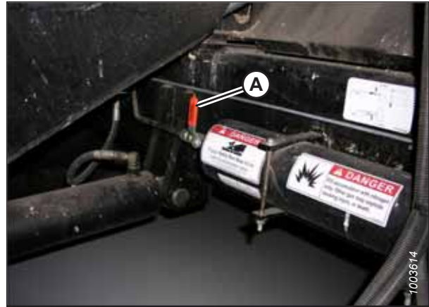
Figure 4.82: Combine Accumulator ON/OFF Switch
