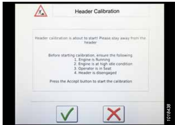
Figure 4.107: Header Calibration Warning
