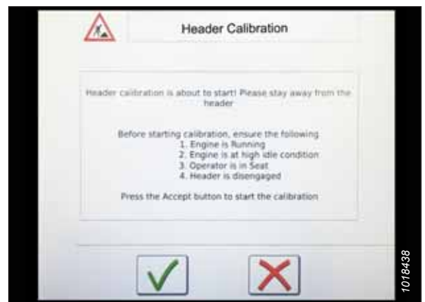
Figure 4.133: Header Calibration Warning
