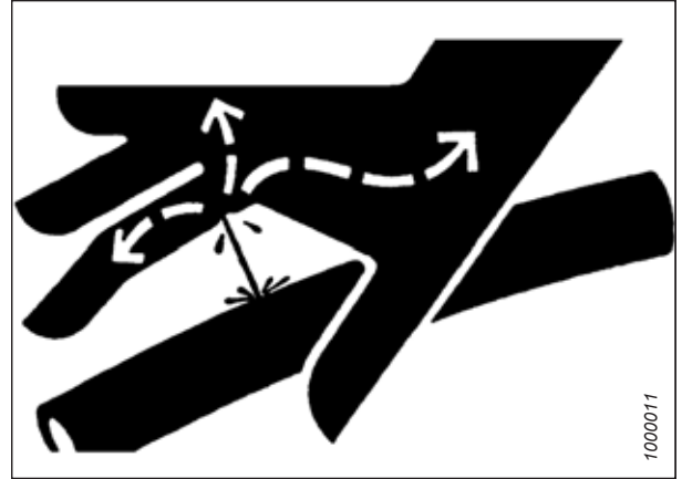
Figure 5.187: Hydraulic Pressure Hazard
