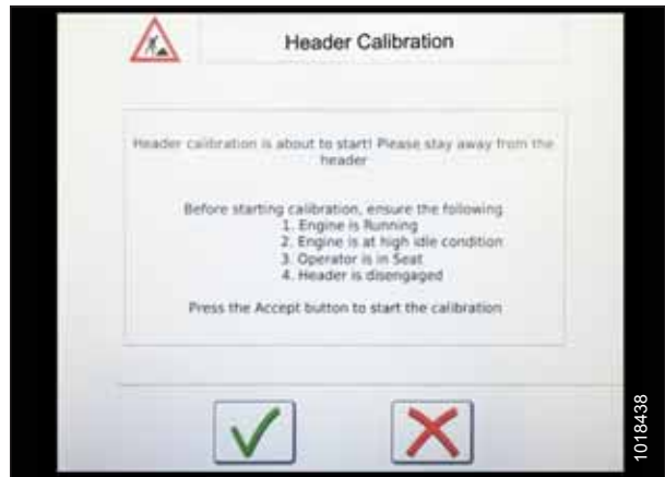
Figure 4.41: Header Calibration Warning
