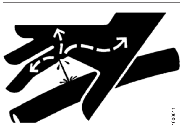
Figure 5.195: Hydraulic Pressure Hazard
