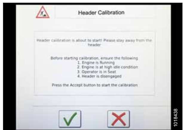
Figure 4.133: Header Calibration Warning
