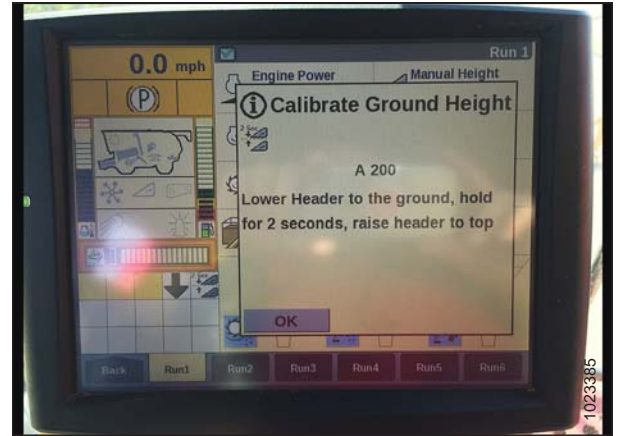
Figure 4.34: Calibrating Auto Header Height
