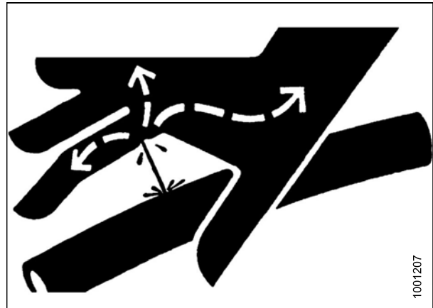
Figure 1.12: Hydraulic Pressure Hazard
