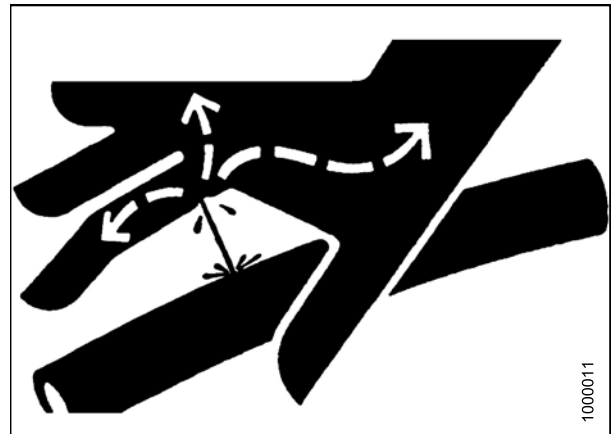
Figure 5.188: Hydraulic Pressure Hazard
