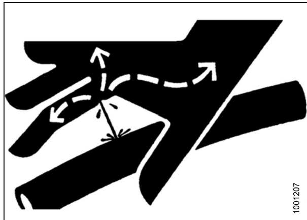
Figure 1.12: Hydraulic Pressure Hazard
